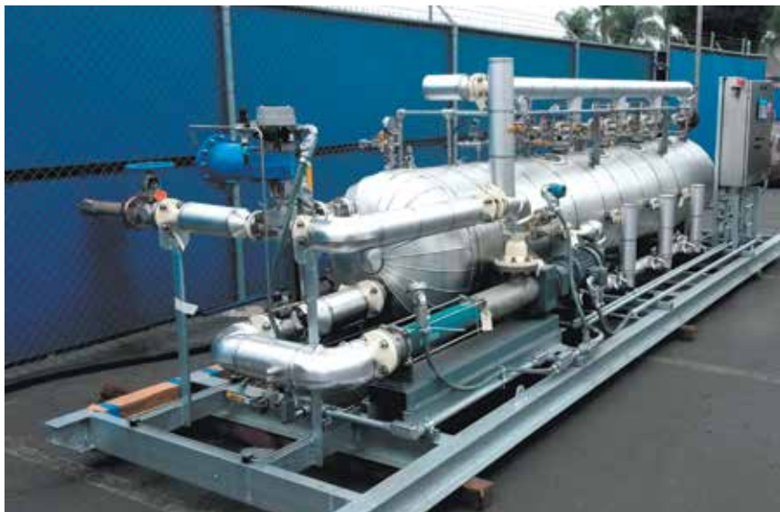
The horizontal design of the degasifier allows use at installations with height restrictions.
