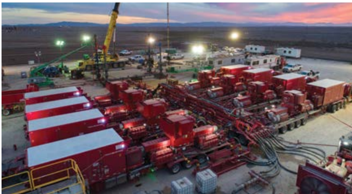
Halliburton says its Zeus electric pumping unit is capable of achieving sustained activity at 5,000 hhp. (Source: Halliburton)
