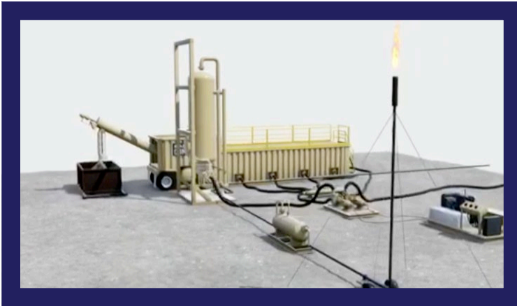
The Sand Commander was designed by CP Energy Services to address both flowback issues and water reuse in one unit. Watch this clip to learn more. (Source: CP Energy Services)
