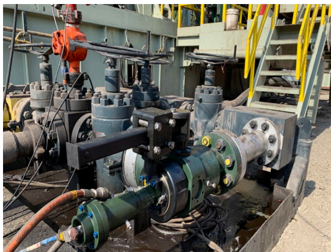
CORTEC's CX-HB3.0 Hydra-Balance Choke and Panel System is a hydraulic dual choke unit that can be controlled via a compact remote panel, which is installed in close proximity to the driller. (Source: CORTEC)
