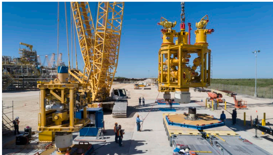
The 275,000-lb capping stack is lifted by a crane during a full-scale mobilization exercise conducted at MWCC’s Texas Deployment Facility in October 2020. (Source: MWCC)
