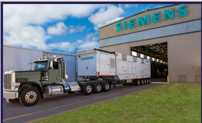
The Via portfolio of 5.8-MW and 7.9-MW class mobile power units provide scalable and rapid mobility solutions for power generation in a variety of oil and gas applications. (Source: Siemens)
